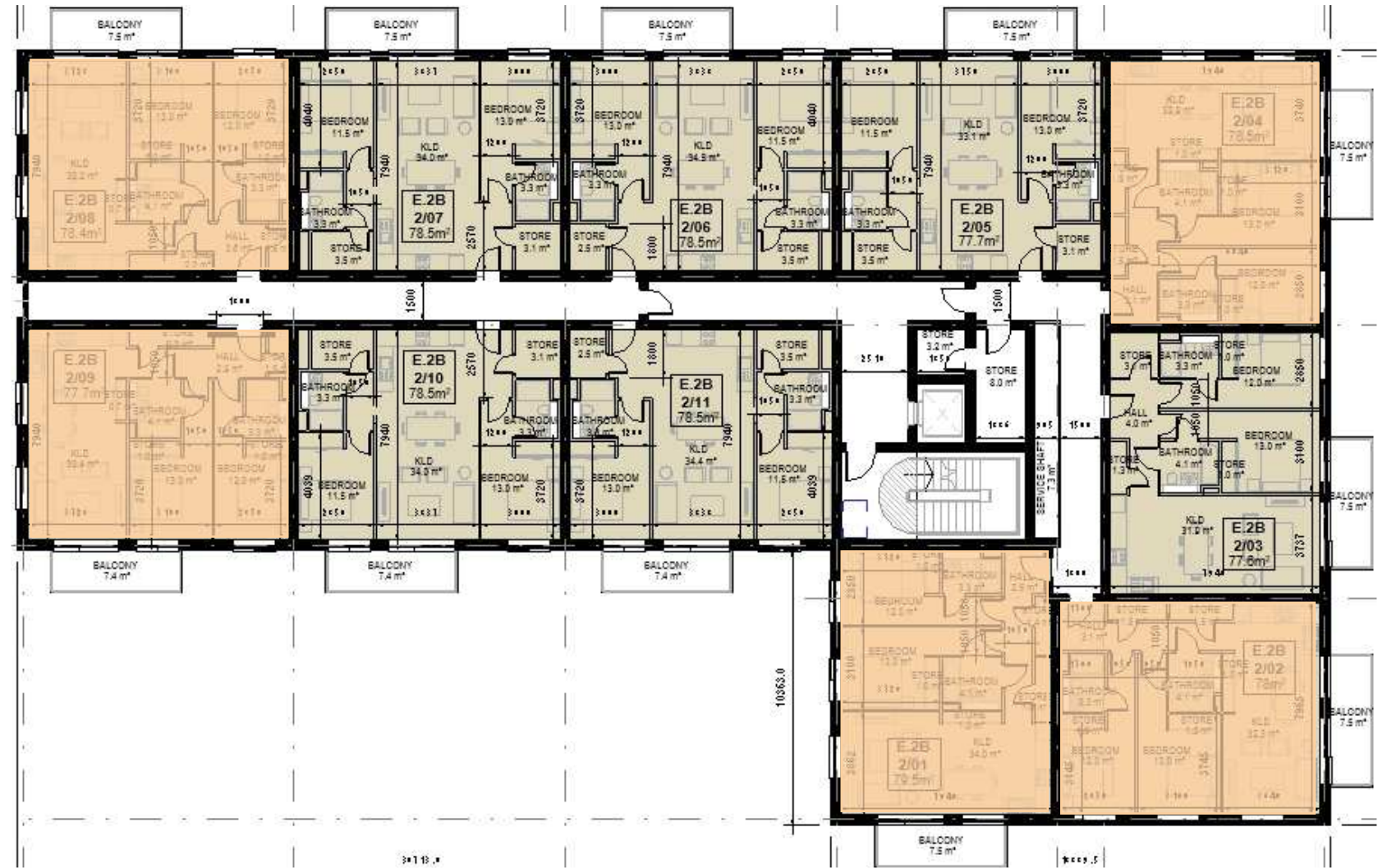
Typical Floor Layout showing Dual Aspect Units
